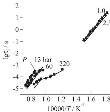
**Figure 4** Ignition delays of *n*-hexane–air mixture within experimental ranges of pressure and temperature tested in available literature. Experiments at 1 and 2.5 bar correspond to present data for the stoichiometric mixture; experiments at 13, 60, and 220 bar correspond to fuel-lean mixture with a fuel–air ratio  $\Phi = 0.5$  reported in [3]. Solid curves correspond to the predictions by the overall mechanism
