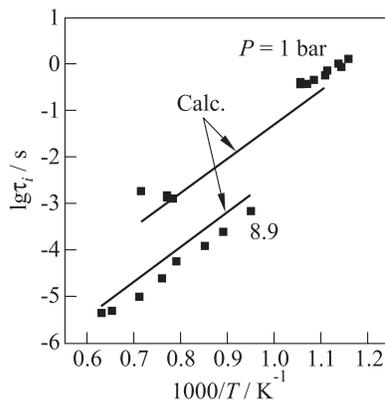
**Figure 6** Ignition delays of the stoichiometric kerosene TS-1–air mixture. Experimental points at 1 bar correspond to present data; points at 8.9 bar correspond to experiments [1] for Jet-A. Solid lines correspond to the predictions by the overall mechanism for the surrogate fuel containing 73% *n*-decane, 9% *n*-hexane, and 18% benzene
