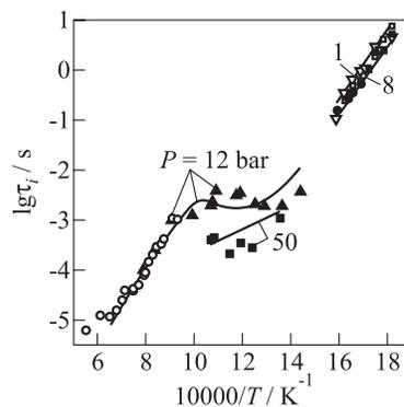
**Figure 3** Ignition delays of the stoichiometric *n*-decane–air mixture within experimental ranges of pressure and temperature tested in available literature. Experimental data at pressures from 1 to 8 bar correspond to present experiments, the data at 12 and 50 bar correspond to [2]; circles correspond to [1]. Solid curves correspond to the predictions by the overall mechanism
