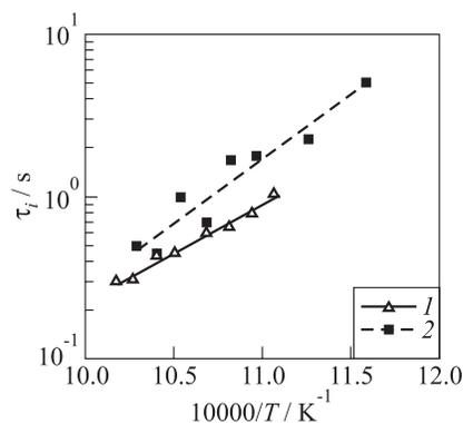
**Figure 2** Comparison of ignition delays of propane–air mixtures measured in the reactor with two different techniques of fuel and air injection: triangles (1) pertain to tests with injection of premixed components, squares (2) are ignition delays measured in tests with separate injection of the fuel and air
