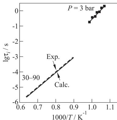
**Figure 5** Ignition delays of the stoichiometric benzene–air mixture. Experiments at 3 bar (squares) correspond to present data; experimental data at 30 to 90 bar (dashed line) are taken from [4]. Solid curves correspond to the predictions by the overall mechanism
