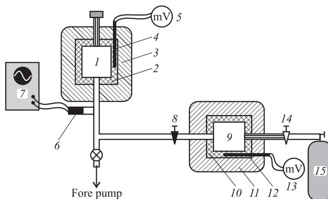
**Figure 1** Schematic of the static apparatus: 1 — reactor, 2 — electrical furnace, 3 — thermal insulation, 4 — thermocouple, 5 — millivoltmeter, 6 — pressure gauge, 7 — recording system including analog-to-digital converter and PC, 8 — fast operating electromagnetic valve, 9 — vessel with mixture, 10 — electrical heater, 11 — thermal insulation, 12 — thermocouple, 13 — millivoltmeter, 14 — valve, and 15 — mixer
