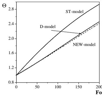
**Fig. 1:** Time history of the mean temperature of a steel particle at  $T_{g\infty} = 1263$  K
