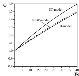
**Fig. 2:** Time history of the mean temperature of a mercury particle at  $T_{g\infty} = 663$  K
