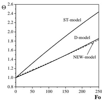
**Fig. 3:** Time history of the mean temperature of a magnesium particle at  $T_{g\infty} = 1600$  K
