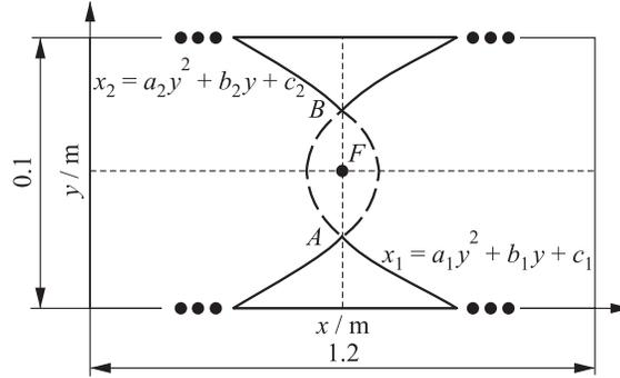
**Figure 1** Schematic of shaped parabolic obstacles in the 2D channel
