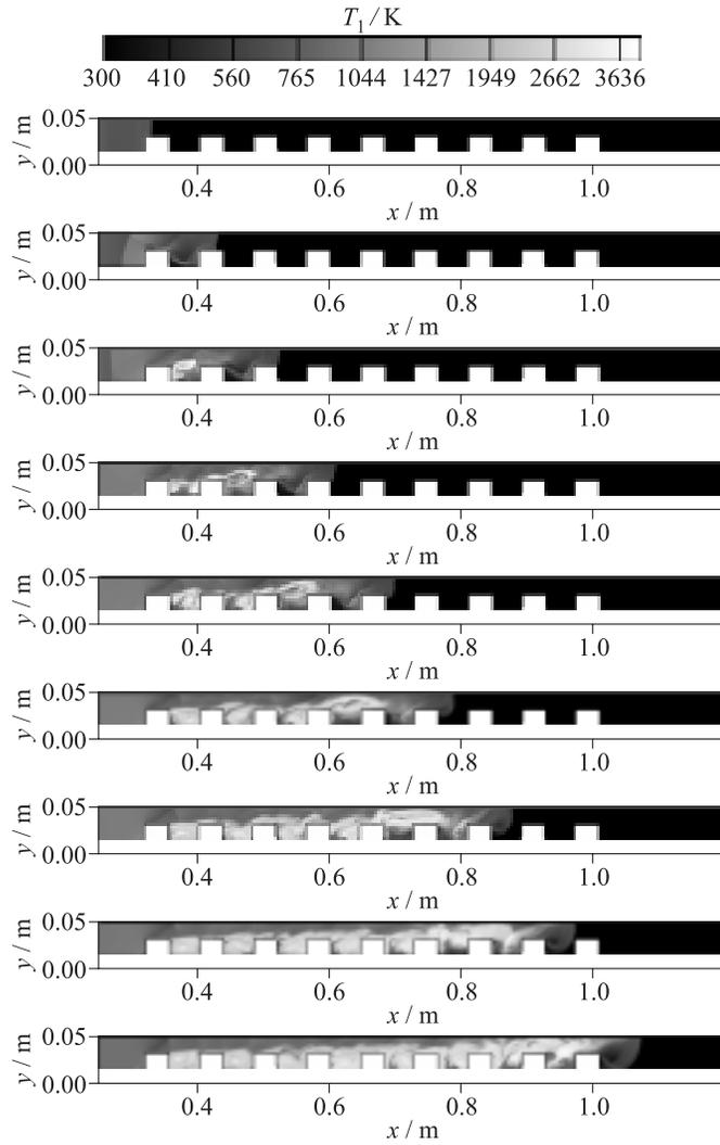
**Figure 3** Snapshots of temperature fields in the channel with regular orifice plates. The upper snapshot corresponds to a time instant of  $80 \mu\text{s}$ . All other snapshots are plotted with time interval of  $100 \mu\text{s}$
