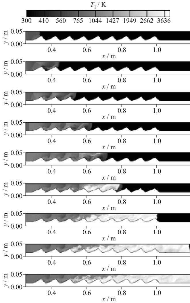
**Figure 2** Snapshots of temperature fields at SDT in the channel with regular parabolic obstacles. The upper snapshot corresponds to time instants of  $80 \mu\text{s}$ . All other snapshots are plotted with time interval of  $100 \mu\text{s}$
