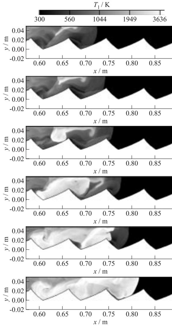
**Figure 4** Evolution of temperature field after gas autoignition above the fifth parabolic obstacle. The upper snapshot corresponds to the time instant of  $590 \mu s$ . All other snapshots are plotted with time interval of  $20 \mu s$
