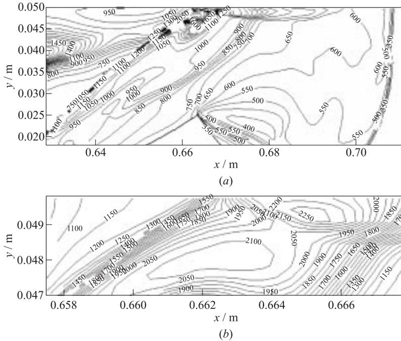
**Figure 5** Predicted temperature isolines in the vicinity of the exothermic center where ignition occurs at  $490 \mu\text{s}$ . The isolines correspond to a time instant of  $470 \mu\text{s}$ : (a) complete temperature field, and (b) explosive view of the temperature field near the exothermic center
