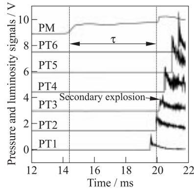
**Figure 5** Records of pressure transducers PT1 to PT6 and photomultiplier (PM) in the test of Series 2a with the SW arrival delay time  $\tau = 5-6$  ms (see curve 13 in Fig. 3)
