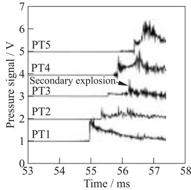
**Figure 4** Records of pressure transducers PT1 to PT5 in the test of Series 2a with the SW arrival delay time  $\tau = 12.2$  ms (see curve 7 in Fig. 3)
