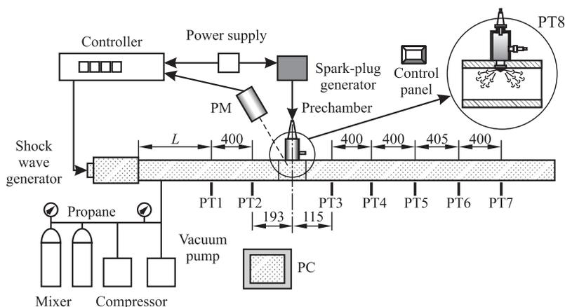
**Figure 1** Schematic of the experimental setup. Dimensions are in millimeters
