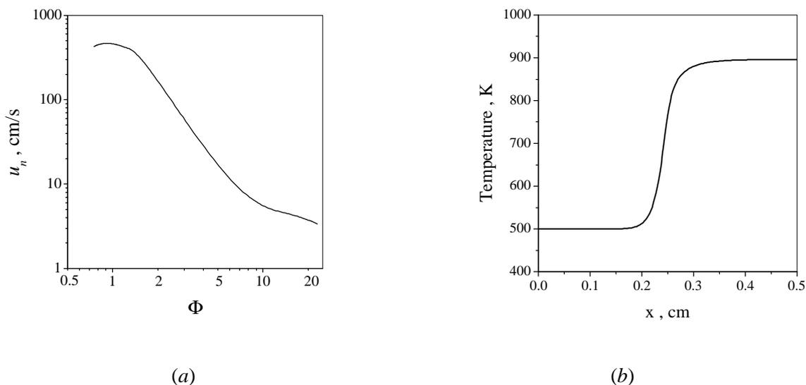
**Figure 5:** (a) Predicted laminar burning velocities of  $n\text{-C}_4\text{H}_{10}\text{-O}_2$  mixtures as a function of equivalence ratio  $\Phi$  at  $T_0 = 500$  K and  $p_0 = 4.1$  bar; (b) Calculated temperature profile in the  $n\text{-C}_4\text{H}_{10}\text{-O}_2$  laminar flame at  $\Phi = 23$  at  $T_0 = 500$  K and  $p_0 = 4.1$  bar
