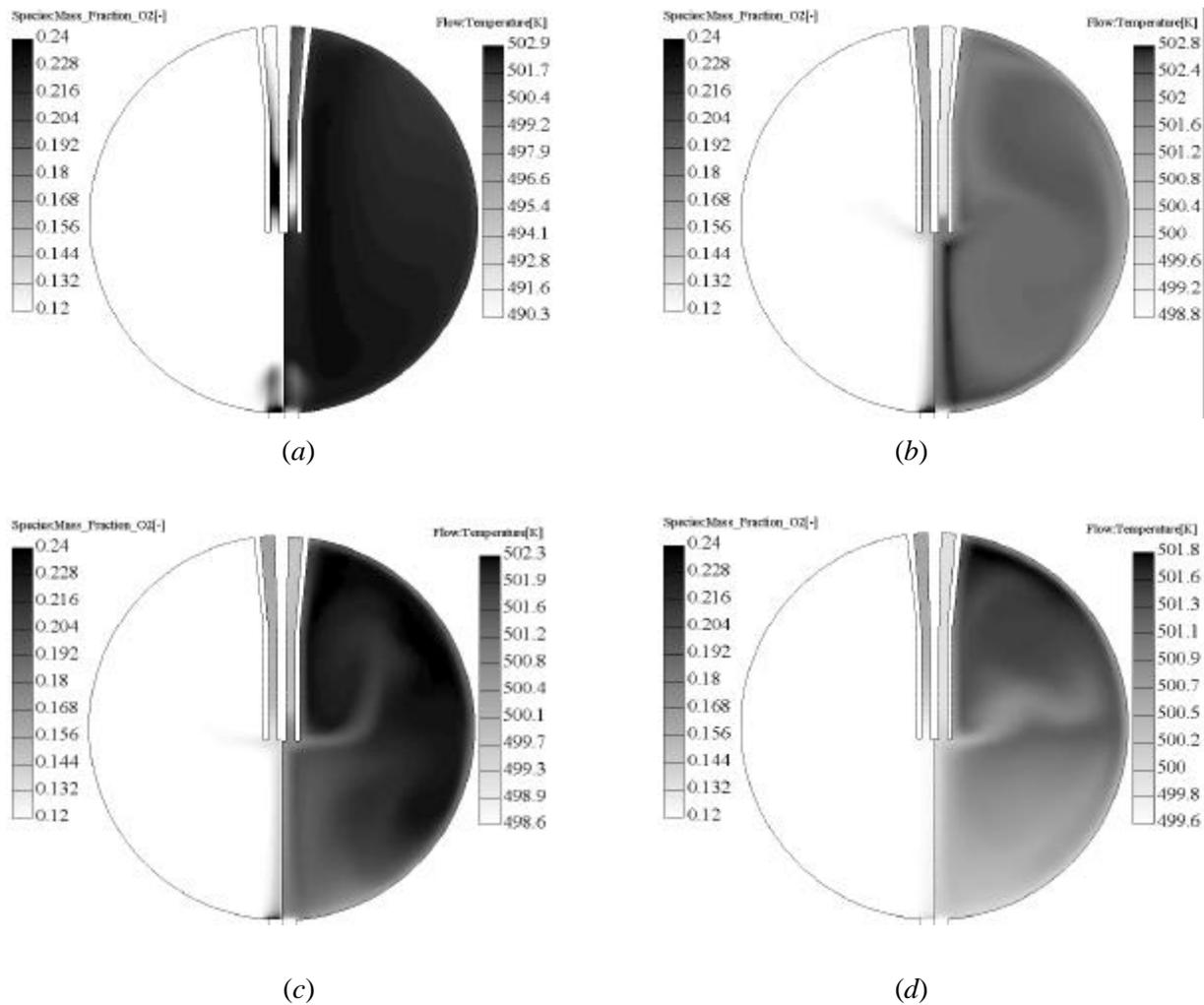
**Figure 4:** Calculated isolines of oxygen mass fraction (left hemisphere) and temperature (right hemisphere) at time (a) 3 s; (b) 10; (c) 20; and (d) 100 s after oxygen injection termination. Initial oxygen pressure was 29.67 bar. Initial *n*-butane pressure was 3.2 bar. Injection duration was 0.01 s
