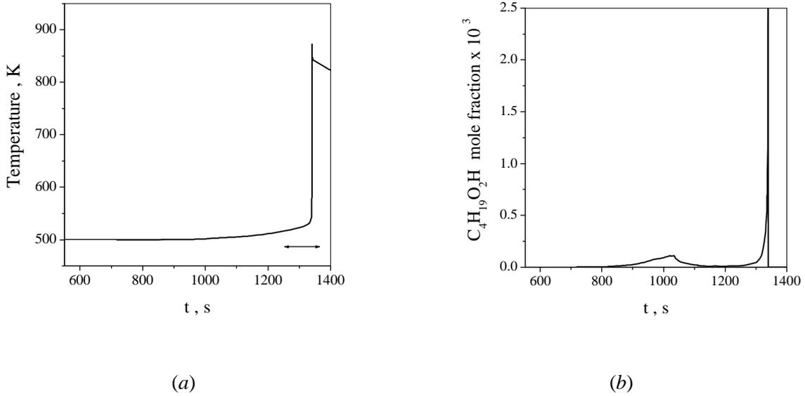
**Figure 6:** (a) Predicted temperature history in the 78% $C_4H_{10}$  +22% $O_2$  test mixture in the course of self-ignition at  $T_0 = 500$  K and  $p_0 = 4.1$  bar (arrow shows the experimental self-ignition delay); (b) Predicted time history of butyl hydroperoxide mole fraction in the test mixture
