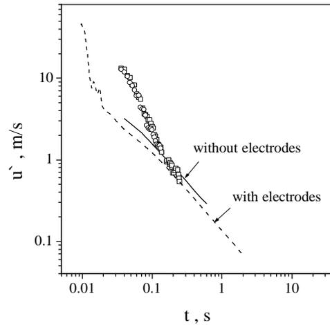
**Figure 1:** Comparison of predicted and measured [1] root-mean-squared velocity fluctuations  $u'$  in the vessel center. Initial oxygen pressure is 21 bar. Initial *n*-butane pressure is 0.4 bar. Injection duration is 0.0117 s. The solid line corresponds to calculations [3]. The dashed curve corresponds to present calculations
