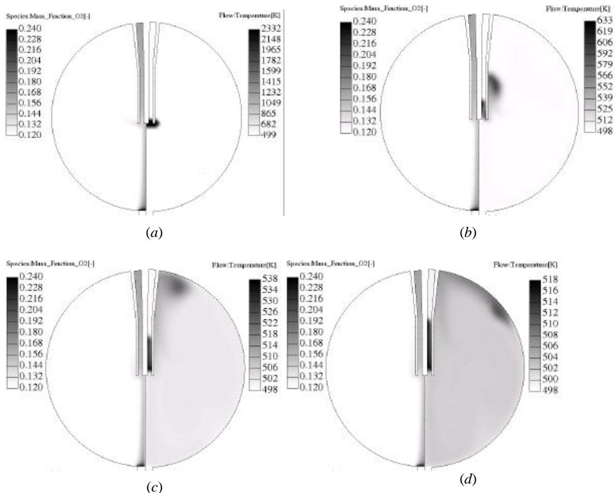
**Figure 7:** Calculated fields of oxygen mass fraction (left hemisphere) and temperature (right hemisphere) after ignition of test mixture in the vessel center 10 s after termination of oxygen injection: (a) ignition completion; (b) 0.3 s; (c) 1; and (d) 2 s after ignition. Initial oxygen pressure in the canister is 29.67 bar. Initial *n*-butane pressure in the vessel is 3.2 bar. Injection duration is 0.01 s. The interval between the isolines is uniform
