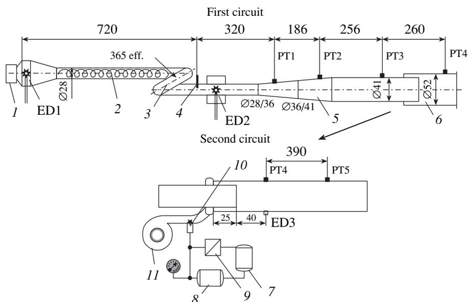
**Fig. 1.** Two-circuit pulse detonation engine demonstrator: (1) air-assist atomizer, (2) Shchelkin spiral, (3) tube coil, (4) ionization probe, (5) conical transition section, (6) second-circuit tube, (7) second-circuit fuel tank, (8) fuel pump, (9) fuel valve, (10) atomizer, and (11) compressor. The sizes are given in millimeters.
