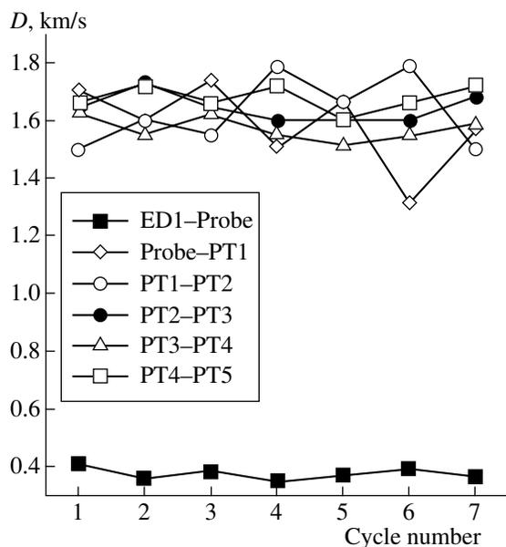
**Fig. 2.** Blast wave velocities  $D$  measured at various measurement segments in the first and second circuits during the operation of the demonstrator in the detonation mode at a pulse repetition frequency of 2.2 Hz.
