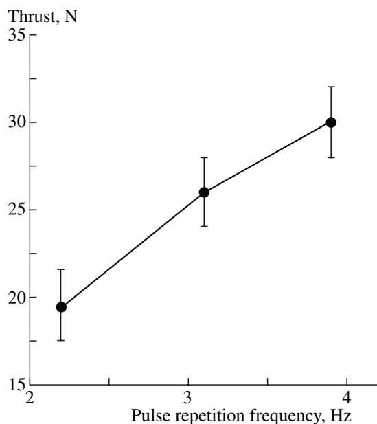
Fig. 3. Measured jet thrust versus pulse repetition frequency.
