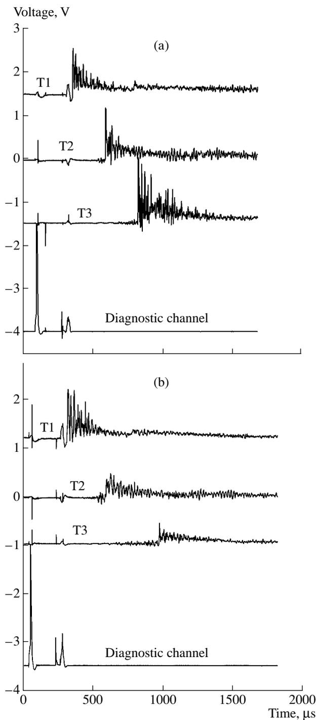
**Fig. 2.** Pressure oscillograms upon (a) detonation and (b) lack of detonation in the spray of *n*-hexane in air. The tube diameter was 28 mm. Detonation was initiated by two successive electric discharges.
