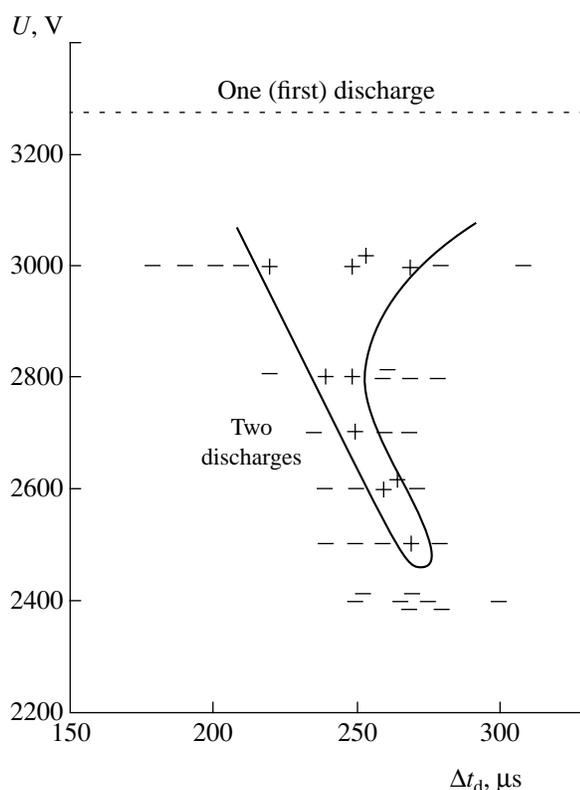
**Fig. 1.** Detonation peninsula for an *n*-hexane spray in air in a tube of 51 mm in diameter when detonation is initiated by two successive electric discharges.
