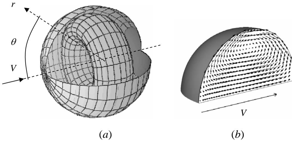
**Figure 1:** (a) Schematic of internal circulation and (b) predicted velocity field in liquid drop with indication of relative values of gas and liquid velocities
