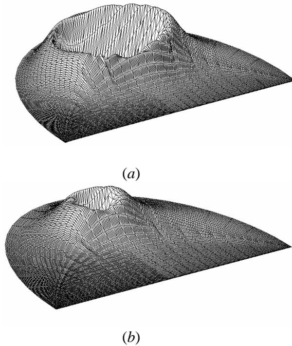
**Figure 6:** Predicted distributions of volumetric vaporization rates in the drop at two subsequent time instants (a) and (b) at the late stage of drop heating with  $\omega = 10^{-2}$
