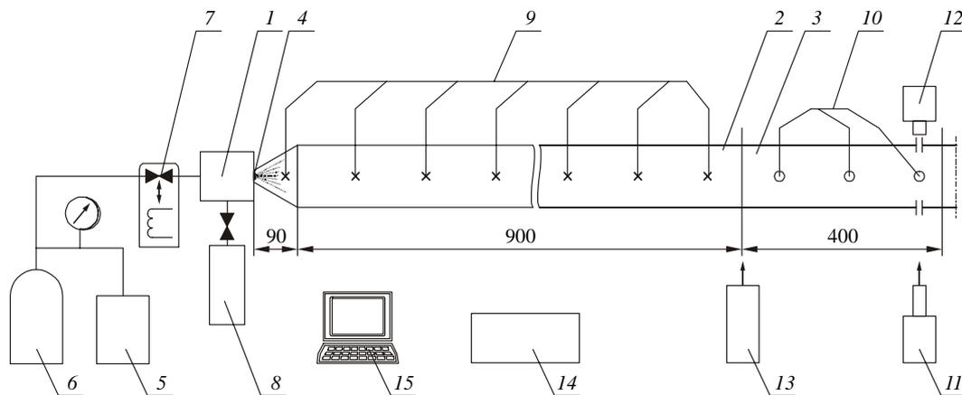
**Figure 3:** Experimental setup for detonation initiation in fuel spray – air mixtures [14–17]. 1 – air-assist liquid-fuel atomizer, 2 – booster section, 3 – test section, 4 – cone, 5 – compressor, 6 – bottle, 7 – solenoid valve, 8 – fuel tank, 9 – igniters, 10 – pressure transducers and ionization probes, 11 – laser, 12 – optical system, 13 – droplet sizing unit, 14 – controller, and 15 – PC. Dimensions in mm
