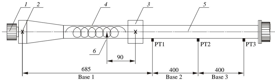
**Figure 6:** Experimental setup with 28-millimeter tube and Shchelkin spiral between two dischargers [17]: 1 — air-assist liquid-fuel atomizer, 2 — first discharger, 3 — second discharger, 4 — Shchelkin spiral, 5 — tube, and 6 — sensor; PT1, PT2, and PT3 stand for pressure transducers. Dimensions in mm
