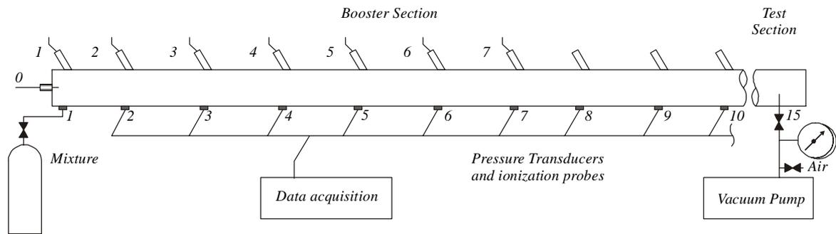
**Figure 1:** Experimental setup for detonation initiation in gaseous fuel–air mixtures [12, 13]. A relatively weak primary shock wave generated by electric dischargers 0 and 1 is amplified to detonation intensities by triggering dischargers 2, 3, 4, etc. in phase with SW arrival at their position
