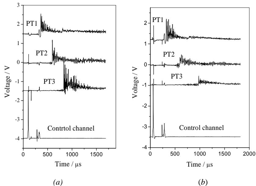
**Figure 5:** Samples of pressure records with (a) successful detonation initiation (time delay between two discharges of  $214 \mu\text{s}$ ), and (b) initiation failure (time delay of  $211 \mu\text{s}$ )
