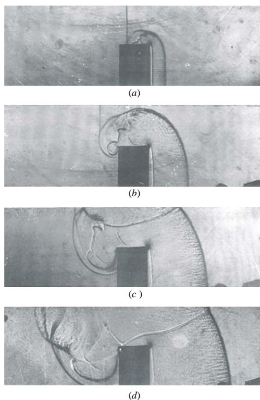
**Figure 7:** Spark Schlieren photographs for obstacle-induced detonation initiation in  $C_2H_4 + 3O_2 + 12Ar$  mixture (initial SW Mach number  $M = 3.2$ , initial pressure 0.053 atm, 20  $\mu s$  frame interval) [23]. The primary SW propagates from right to left.
