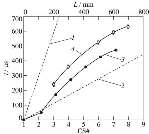
**Figure 2:** Experimental distance–time diagram of shock wave amplification in the stoichiometric  $C_3H_8$ –air mixture. Detonation occurs after cross-section CS7 [12, 13]. 1 – slope of sound velocity, 342 m/s, 2 – slope of detonation velocity, 1800 m/s, 3 – triggering timing of dischargers in various cross-sections, and 4 – shock wave arrival timing
