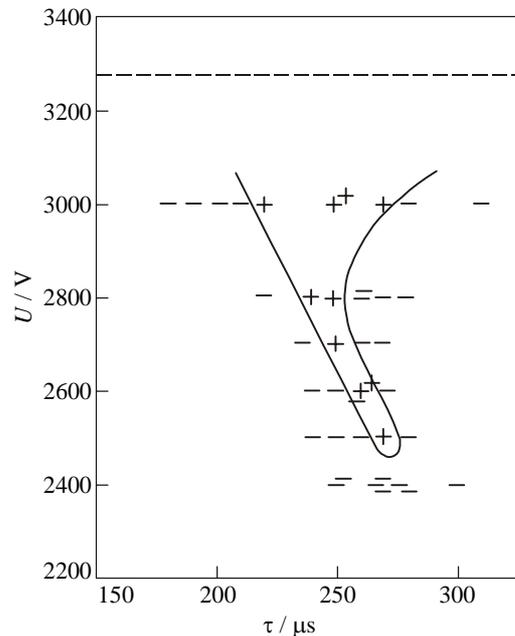
**Figure 4:** Measured dependency of detonation initiation energy (in terms of voltage  $U$  applied to high-voltage blocks of two dischargers with similar capacitance of  $300 \mu\text{F}$ ) vs. the delay time  $\tau$  of the second discharger triggering (counted from activation of first discharger) [14–17]. Tube diameter 51 mm. Dashed line shows voltage required for detonation initiation by a single discharger of capacitance  $2 \times 300 \mu\text{F} = 600 \mu\text{F}$ .
