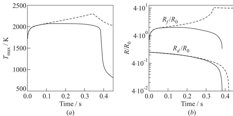
**Figure 1** Comparison of flame temperature (a) and dimensionless flame and drop radii,  $R_f/R_0$  and  $R_d/R_0$ , histories for the isolated drop (solid curve) and drop in suspension (dashed curve,  $\Phi = 1.1$ ). Fuel: *n*-heptane, Oxidizer: air, Initial pressure and temperature: 0.1 MPa and 300 K;  $R_0 = 0.25$  mm.
