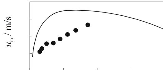
**Figure 7** The comparison of predicted and measured<sup>4</sup> limiting approach stream velocities for bluff-body stabilized combustion of methane as a function of fuel mass flow rate
