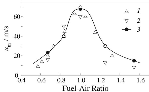
**Figure 4** Comparison of predicted (3) and measured<sup>2,10</sup> (1, 2) limiting approach stream velocities depending on the fuel-air ratio
