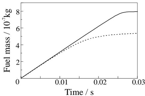
**Figure 6** The predicted history of mixture fraction (solid curve) and fuel mass (dashed curve) in the burner at  $m_g = 30$  mg/s,  $u_{in} = 15$  m/s, and  $x_{jc} = 26$  cm
