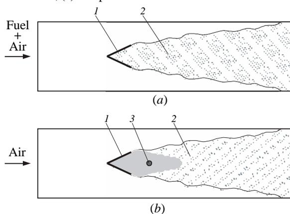
2 — combustion products, 3 — fuel injection core
