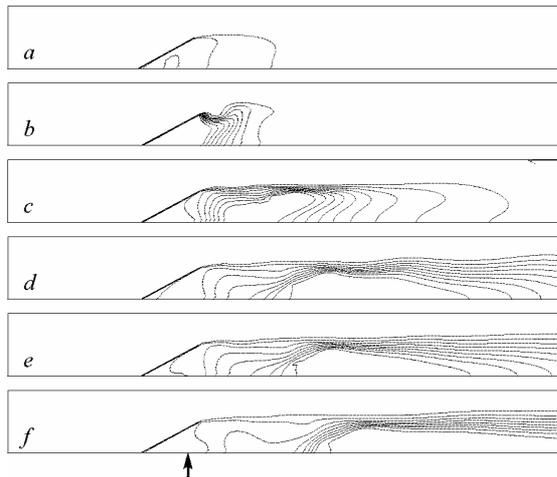
**Figure 5** Predicted temperature fields during non-premixed combustion of methane-air mixture in a burner with flame holder. Temperature fields correspond to  $t > 70$  ms after ignition and  $u_{in} = 10$  m/s. Arrow shows a position of fuel injection core. (a)  $m_g = 2$  mg/s, (b) 15, (c) 20, (d) 50, (e) 100, (f) 200
