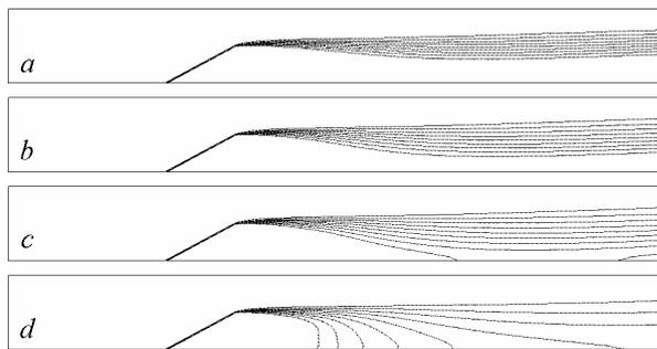
**Figure 2** Predicted temperature fields during combustion of premixed stoichiometric methane – air mixture in a burner with flame holder:  $t = 50$  ms,  $u_{in} = 40$  m/s (a), 50 (b), 60 (c), and 80 (d)
